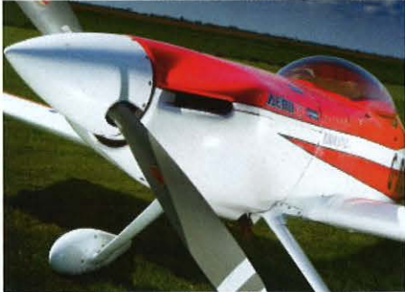
Massive 80in-diameter c/s propeller leads the way.
