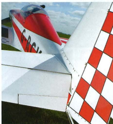
Tail surfaces are standard Van's RV4.
